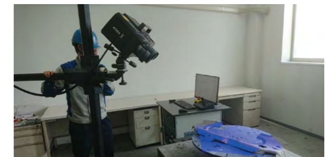
Measurement using an image-based non-contact measuring machine
